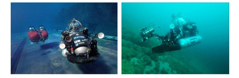
The one-atmosphere **DeepWorker 2000** submersible allows a pilot to go deeper and spend more time below the surface than traditional diving methods. The compact and lightweight **DeepWorker 2000** is easy to operate and can be piloted with minimal training. Horizontal and vertical thrusters give unparalleled manoeuverability; the **DeepWorker 2000** can hover and 'fly' underwater. **DeepWorker 2000** is available in a 3300ft (1000m) configuration as a **DeepWorker 3000**.
